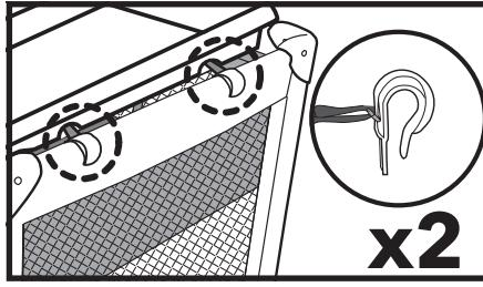
2. Press release button on each end of the metal support bar that holds the straps with 'C'-clips in place.
