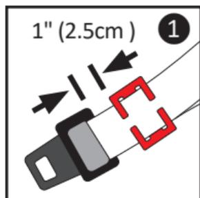
Test installation to see if child restraint is secure. The child restraint should **NOT** be able to move in any direction where it connects to the vehicle. If the child restraint can be moved more than 1 inch (2.5 cm) in any direction at the connection point, then unbuckle the seat completely and repeat the steps above until secure (see “Installation safety check”). If you have any questions, please contact Harmony Juvenile Products customer service.
