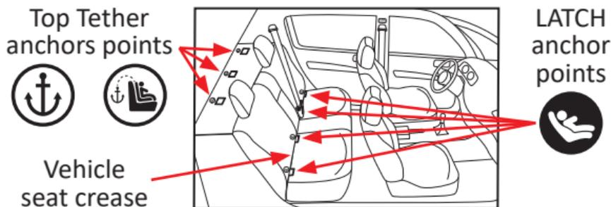
**! WARNING:** CONSULT YOUR VEHICLE OWNER'S MANUAL FOR THE EXACT PLACEMENT OF THESE ELEMENTS IN YOUR VEHICLE, AND FOR MAXIMUM LATCH WEIGHT ALLOWANCES PRIOR TO INSTALLATION AS SOME MANUFACTURERS HAVE LOWER MAXIMUM WEIGHT ALLOWANCES FOR LATCH USAGE.
