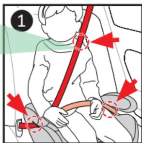
4. Buckle the vehicle seat belt into place and ensure it is secure by gently pulling on it.
