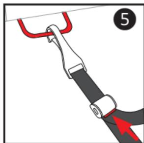
**! WARNING:** NEVER put two LATCH connectors on one vehicle LATCH anchor unless specifically allowed by the manufacturer **6**.
