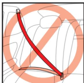
**! NEVER** use a vehicle seat belt system where the lap and shoulder belts have independent retractors.
