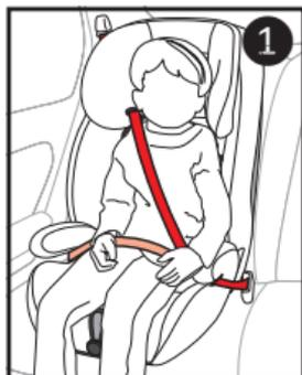
! **WARNING:** Use **ONLY** the vehicle's lap and shoulder belt system when restraining the child in this booster seat. LATCH **WILL NOT** secure your child in the booster seat ①.
