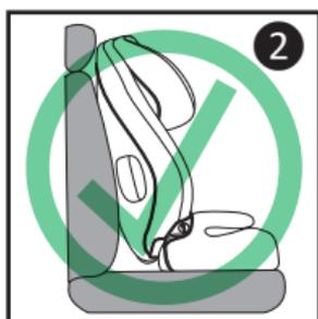
**! WARNING:** Remove the vehicle headrest and/or mesh storage pouch if it inhibits the child restraint from lying flush against the vehicle seat back **3**.
