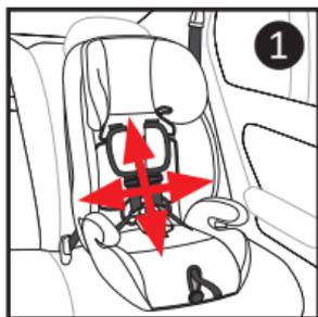
The back of the child restraint (connection point) should not move more than 1 inch (2.5 cm) in any direction.
