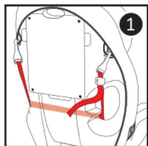
1. Place the child restraint flush against the back of a forward-facing vehicle seat. Adjust the recline as necessary (see “Recline”).
