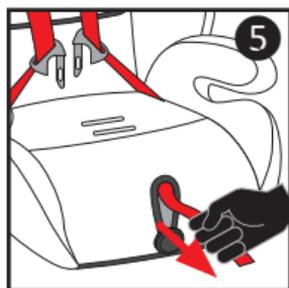
8. Pull the up-front harness adjustment strap as far as it will go. This will lock the splitter plate into the base of the seat **5**.
