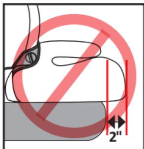
**! DO NOT** use this child restraint in a seating position where the vehicle seat belt or seat belt buckle is not easily accessible with the child restraint secured in place.
