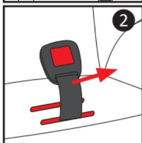
5. Push the buckle upwards through the fabric seat cover.
