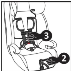
3. Unbuckle harness straps by pressing on the **RED** buckle release button and by pulling the buckle clips out ④. Move harness straps to the side.
