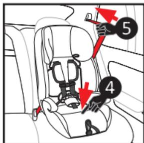
6. The locked seat belt retractor will not allow you to add any length to the belt until you unbuckle the seat belt.
