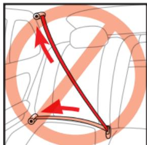
**! NEVER** use a cut, frayed or damaged vehicle seat belt.
