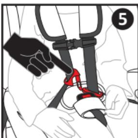
6. Place harness straps over child's shoulders and insert buckle clips into buckle until they 'click' into place ⑤.
