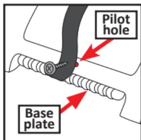
**! Before tightening screw, make sure belt strap is pointing upwards and that the **RED** belt safety guide opening is facing forward. **DO NOT** overtighten screw.**
