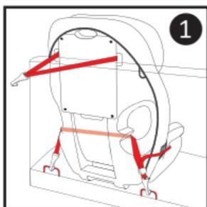
2. Place the child restraint flush against a forward-facing vehicle seat, centered between the LATCH anchors. Adjust the recline as necessary (see "Recline").
