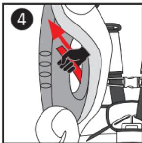
**TIP:** If you are not able to tighten LATCH using the method above, try pulling the LATCH strap up through the belt path (under the fabric) ❹, then tighten.
