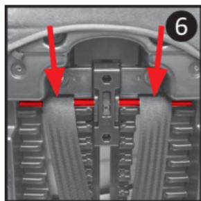
9. Roll strap tightly, secure roll with an elastic band and store rolled strap under the fabric seat cover in the opening of the up-front adjuster.
