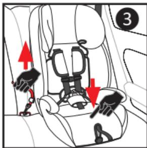
4. Tighten LATCH by placing your knee on the child restraint base and by using your full weight to push the child restraint down as you simultaneously pull upwards on the free end of the adjustment belt ❸.
