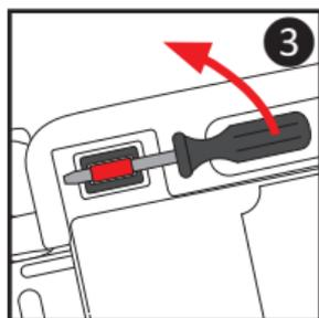
4. Lie child restraint on its side and find the metal locking plate for each harness strap on the underside of the base of the child restraint. Place a screwdriver under the loop of the strap and pry up to unlock the metal locking plate from the plastic base **3**. Turn each metal plate so that it can slide up and out through the plastic seat base.
