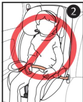
! **NEVER** use a vehicle lap-only belt to secure child in booster seat ②.
