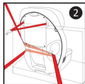
3. Buckle the vehicle seat belt. The vehicle seat belt **MUST NOT** be twisted.
