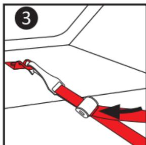
**! WARNING:** Ensure that Top Tether strap is **NOT** twisted.
