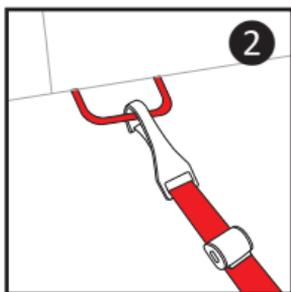
3. Fasten LATCH hooks to vehicle lower anchors ensuring the hooks are facing downwards ❷. Pull firmly to be sure that they are attached. **BELT MUST LAY FLAT AND NOT BE TWISTED.**
