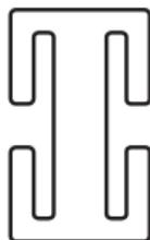
If your vehicle’s 3-point lap-and-shoulder seat belt is equipped with an Emergency Locking Retractor (ELR) that is **NOT** convertible to function as an Automatic Locking Retractor (ALR), then the locking clip **MUST** be used.
