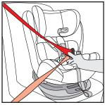
base positioning guide **ON THE SAME SIDE** as the seat belt retractor. Replace insert cushion.
