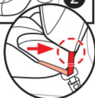
Installation Guide (Parts list - 'J'). See illustrations for proper routing path of the 3-point lap-and-shoulder belt ③.
